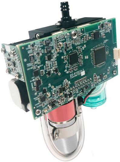
The 9300P-OEM measures up to 30 channels of particle count data from 0.3 to 25.0  $\mu\text{m}$  with a flow rate of 1.2 LPM. The assembly is mounted on a plate for ease of integration. The unit includes a particle sensor, particle counter board, integrated vacuum pump and manifold with pre/post filters, real-time clock/calendar with battery backup, logging and data storage for up to 65,000 sample records, communicates via UART and operates from 7-15 VCD.
